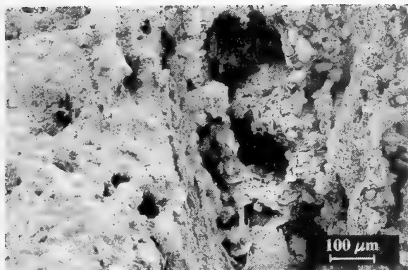
Figure 14. SEM image showing an area of dense limestone adjacent to an area of chalky calcite. The dense limestone contains fewer tubules than the chalky limestone.
